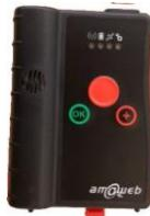
This communication is done in two ways, via voice allowing the RC and the crew to exchange information about reason for retiring, the state of the occupants and via the GPRS communication link, the equipment has with the Rally Control.
