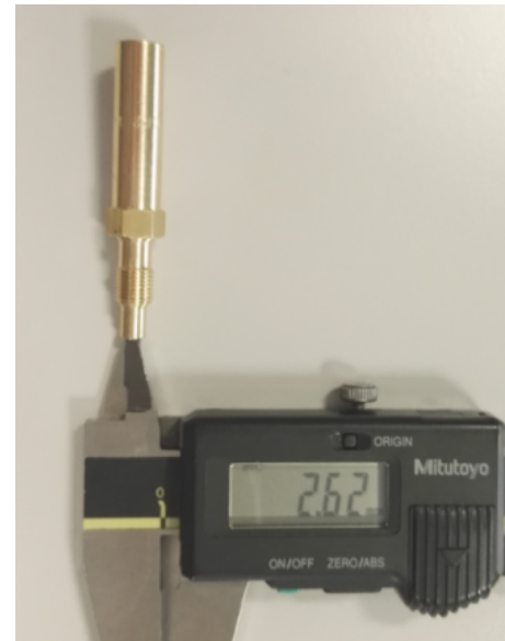
17.10.7) Idle jet Idle jet has to be stamped with 60. Plug gauge 0,65 mm may not enter the bore (use jet gauge set Rotax part no. 281 920).
