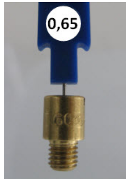
17.10.7) Idle jet Idle jet has to be stamped with 60. Plug gauge 0,65 mm may not enter the bore (use jet gauge set Rotax part no. 281 920).
