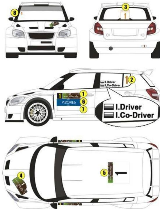
**DOOR PANELS (1)** - Each panel shall be placed horizontally at the leading edge of each front door with the number at the front. The top of the panel shall be between 7 cm and 10 cm below the lower limit of the window.
