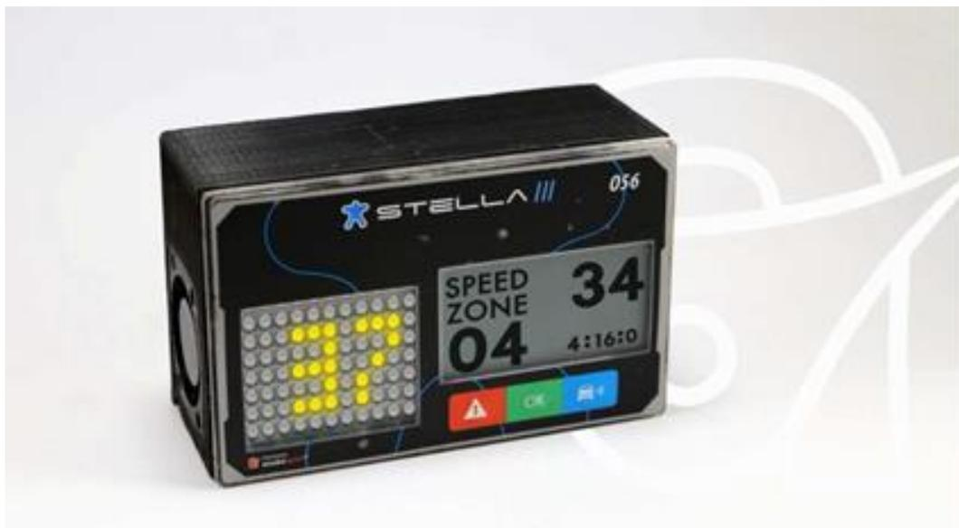
Upon entering the speed zone, the speed limit will change from flashing yellow to steady red color on your LEDS monitor.
