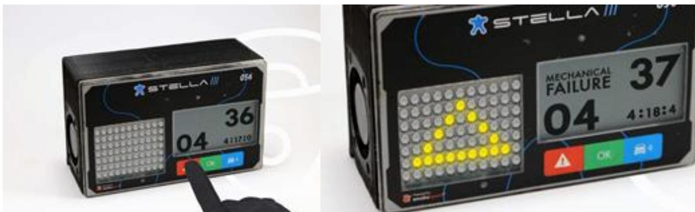
Competitors approaching your vehicle with mechanical failure will receive an alert on their led monitor, a symbol in the shape of flashing red triangle and an alert sound or a beep when they are within 300m of the damaged vehicle.
