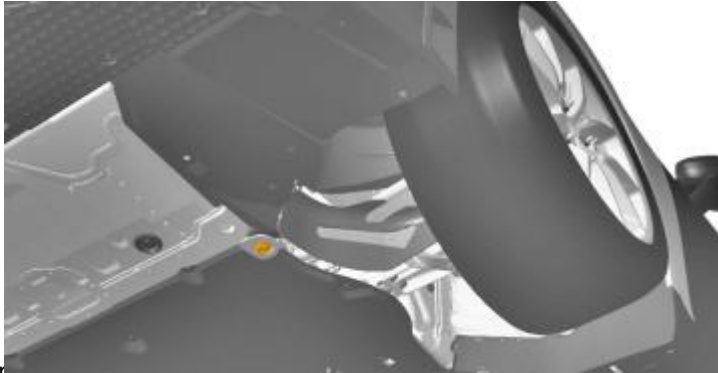
Front ground clearance: 70mm
