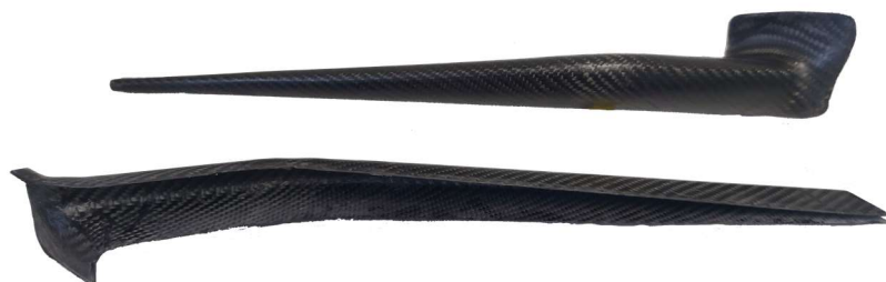
Protection for the floor of the bodywork
