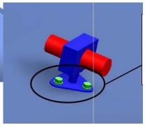
Support: maximum height: 40mm, bounded with screws to a backplate (minimal thickness 3mm). The backplate must be located
