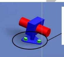
Support : maximum height: 40mm, bounded with screws to a backplate (minimal thickness 3mm). The backplate must be located inside the bodywork, The bodywork must be sandwiched between the support and the backplate.
