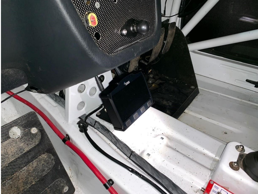
Figure 2. The SAS tracking unit mounted onto the 25mm rubber ball mount and connected through the RallySafe connector
