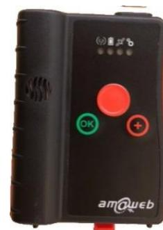
This communication is done in two ways, via voice allowing the RC and the crew to exchange information about the reason for retiring, and the state of the occupants and via the GPRS communication link, the equipment has with the Rally Control.
